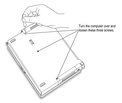
5 Lift up the computer and carefully turn it over to remove the three loosened screws.
